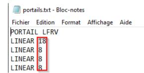
Note: Be careful, the line numbering starts from zero and goes up to 19. For example, if you want to modify the opening time of hangar door 1, you will need to adjust the time on line number 2.
